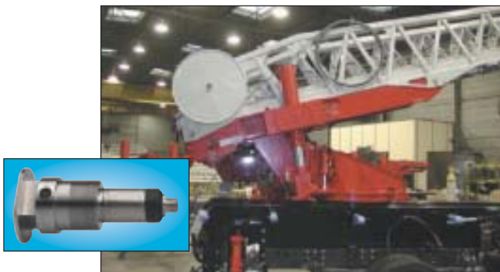
Force measurement to determine the load status on a fire truck turntable ladder
