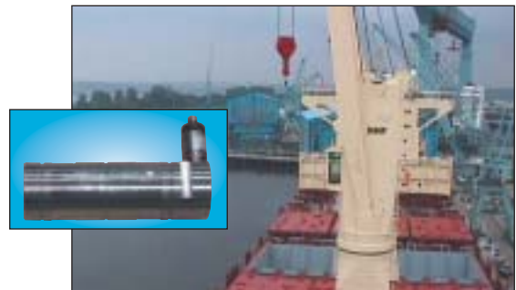
Force measurement for overload protection in the fork bearing of a ship crane"
